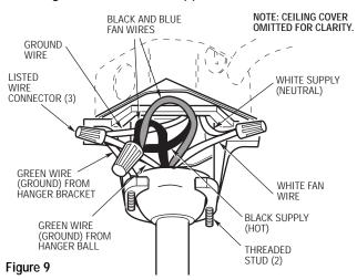
2. Securely connect the fan motor white wire to the supply white (neutral) wire using wire connector supplied (Figure 9). Securely connect the fan motor black wire and blue wire to the supply black (hot) wire using wire connector supplied (Figure 9). After connections have been made, turn leads upward and carefully push leads into the outlet box, with the white and green leads on one side of the outlet box and the black and blue leads on the other side of the outlet box.
